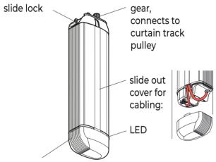
cover: remove to access connector-area and basic controlling buttons
